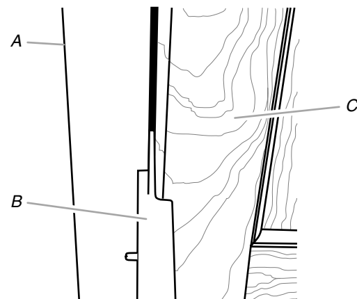
A. Adjacent cabinet B. Installation block C. Panel on door
