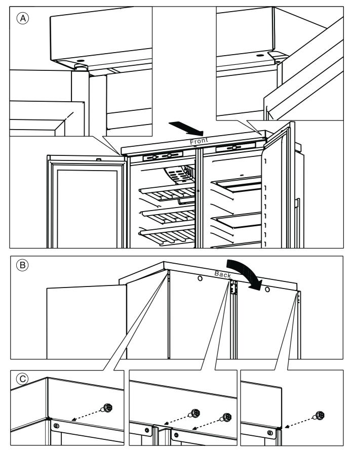
• Fit the trim "II" between the two units by pressing along the entire profile, see figure below.
