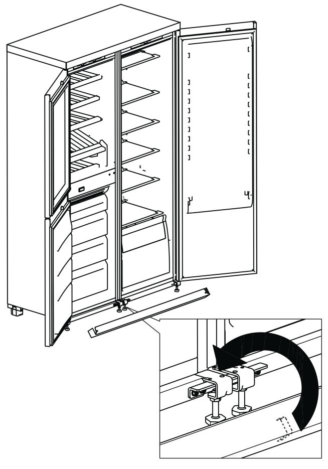
• Fix the front of the top and kickplate with M5x12 screws (bag  $\ll$ 1»).
