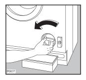
Unscrew and remove the filter.
