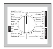
The selector dial can be turned either clockwise or anticlockwise to select the required wash programme.
