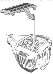
IMPORTANT! If the temperature rises above -5°C (23°F) or 0°C (32°F) respectively the machine MUST be restored to its normal set-up. Otherwise there is a risk of overheating, which can cause severe engine damage.
