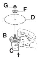
Fit the nut (G). The nut must be tightened to a torque of 35-50 Nm (3.5-5 kpm). Use the socket spanner in the tool kit. Hold the shaft of the spanner as close to the blade guard as possible. To tighten the nut, turn the spanner in the opposite direction to the direction of rotation (Caution! left-hand thread).
