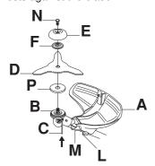
Screw the support cup (E) onto the output shaft threads (CAUTION! Left-hand thread). Tighten to a torque of 35-50 Nm (3.5-5.0 kpm). Use the socket spanner in the tool kit. Note that the locking pin (C) must remain inside the gear housing to lock the drive disk. Hold the shaft of the socket spanner as close to the blade guard/combination guard as possible.
