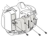
Remove the air filter and air filter cover from the machine. Fit the air filter and air filter cover supplied with the winter kit.
