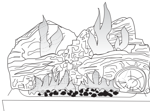
Figure 18. Proper flame picture.
