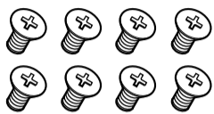
Flat countersunk screws (M5 x 8 mm)
