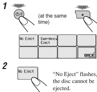
“No Eject” flashes, and the disc cannot be ejected.
