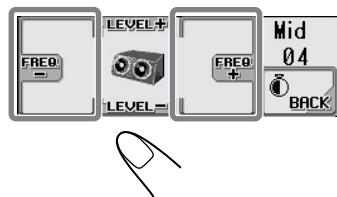
**Low:** Frequencies higher than 55 Hz are cut off to the subwoofer.
