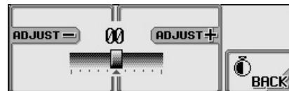
Adjust the balance—speaker output balance between the left and right speakers.
