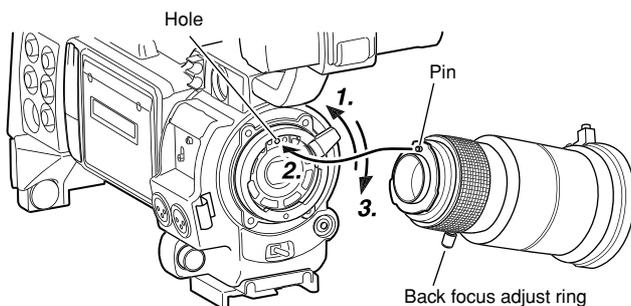
1. Loosen the mount ring of the camcorder.
