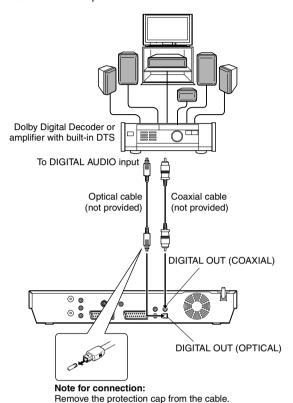
Connect the unit and a Dolby Digital decoder or an amplifier with built-in DTS using either an optional optical cable or an optional coaxial cable.
