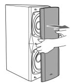
**To attach the speaker grille,** put the projections of the speaker into the holes of the speaker grille.
