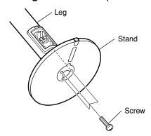
Do not tighten each screw completely one by one.
