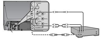
Note that the connection with a video cable will be ignored in case you connect a VCR to the TV with both video cable and S-VIDEO cable.
