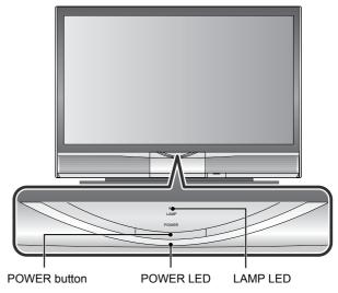
When the POWER button is pressed, the POWER LED lights up and the LAMP LED indicator blinks in orange for approximately 1 minute at approximately every 2 seconds. As the picture becomes brighter, the LAMP LED goes out.
