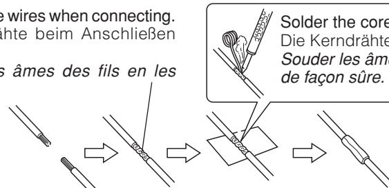
Solder the core wires to connect them securely.
