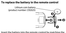
Insert the battery into the remote control by matching the polarities (+ and -) correctly
