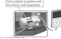
To detach the dock adapter from the dock ush the slot and pull p to remove the dock
