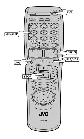
Your remote control can operate the basic functions of your satellite tuner set. In addition to JVC satellite tuners, other manufacturer's satellite tuners can also be controlled by setting the appropriate switch on the remote control.
