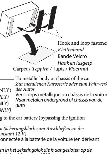
Remove the backing from the hook and loop fastener and attach it to the bottom of the unit. Install the Smartphone Adapter unit on the carpet.
