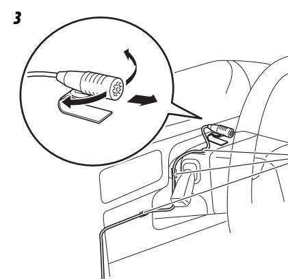
Secure the microphone cord using cord cramps (not supplied) if necessary.
