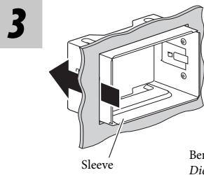
Bend the appropriate tabs to hold the sleeve firmly in place.
