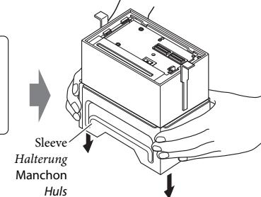
When you stand the unit, be careful not to damage the fuse on the rear.
