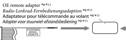
Steering wheel remote controller (equipped in the car)
