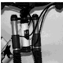
Proper Cable Routing
