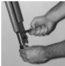
Removing Air Damper
