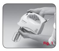
Insert the beaters by pushing the shaft of the socket, turning slightly if required until they lock into place.
