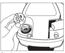
**Step 3** Check oil level. Oil level should always be between the "FULL" and "ADD" marks on the dipstick. Be sure the machine is level when checking the oil level. (Refer to the engine's operating manual for seasonal grades.)
