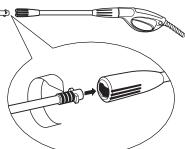
**Step 2** Insert the spray wand of your choice into the wand extension. Press in against the spring tension and twist into the locked position.
