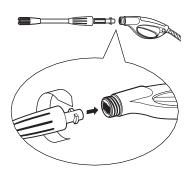
**Step 2** Slide the wand extension into the gun. Turn the wand collar onto the gun threads until tight.
