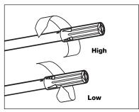
Turn the wand nozzle clockwise to high, for pressure cleaning. Turn the nozzle counter clockwise to low, for detergent application.
