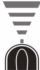
Low pressure fan jet for detergent injection
