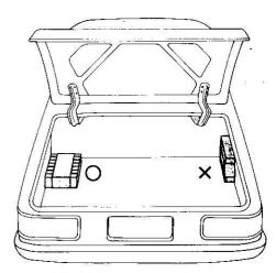
When the installing this unit in the trunk, place it with its heat radiation holes facing upwards to maximize their effect.
