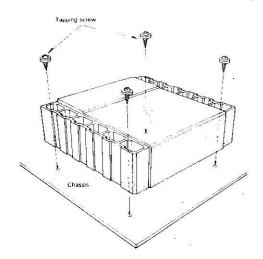
· Use screws supplied as accessories when installing the unit.
