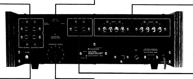
Note: Never set CHANNEL SELECTOR switch to the position other than that intended for use of this amplifier unit.
