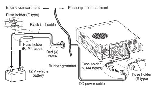
**Note:** If you use the transceiver for a long period when the vehicle battery is not fully charged or when the engine is OFF, the battery may become discharged and will not have sufficient reserves to start the vehicle. Avoid using the transceiver under these conditions.
