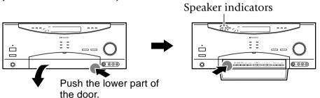
To turn on the front B speakers, press the **SPEAKERS B** key located in the door of the receiver's front panel.
