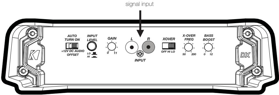
**Automatic Turn-On Selection:** The DX series offers three different automatic turn-on modes that can be selected on the end panel; +12V, DC Offset, and Audio. Using either the DC Offset or Audio mode causes the REM terminal to have +12V out for turning on additional amplifiers.
