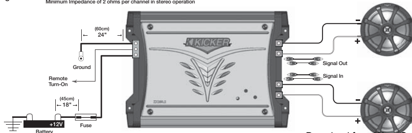
Figure 2 Two Channel Operation (Stereo) Minimum Impedance of 2 ohms per channel in stereo operation
