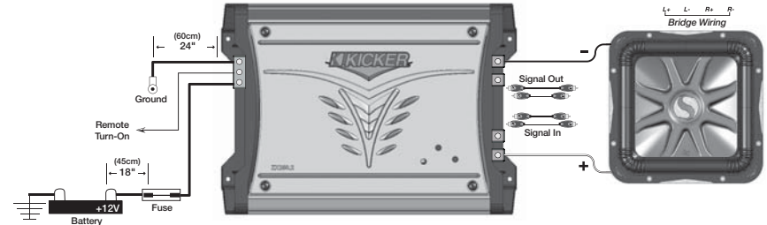
Bridged Operation (Mono) Minimum impedance of 4 ohms while in bridged operation
