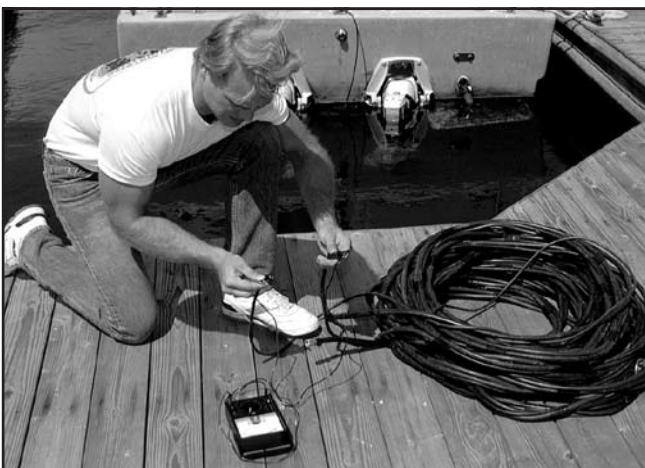
Fig. 8 Preliminary testing of the umbilical with a volt-ohm meter to check for continuity.
