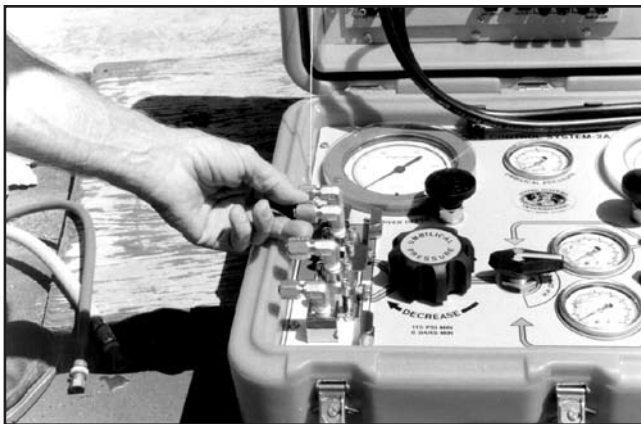
Fig. 11 All of the outlet fittings on the KMACS 5 must be capped prior to storage.
