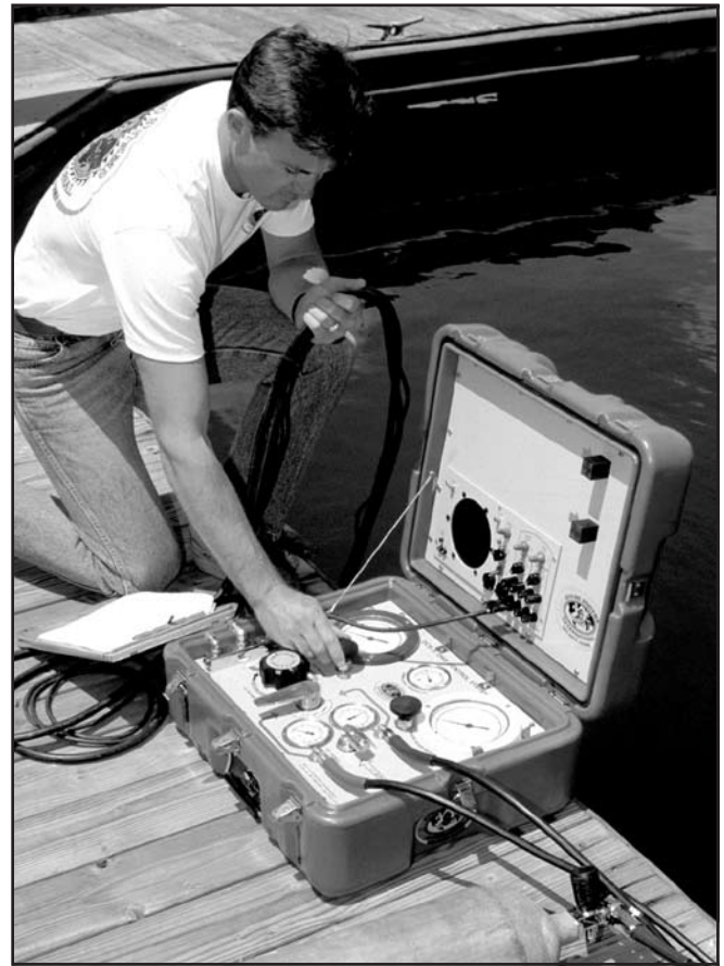
Fig. 10 KMACS 5 operator taking a reading with the pneumo knob. The knob should be turned very slowly.
