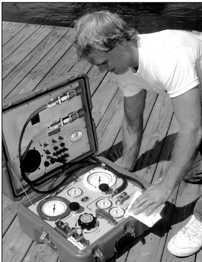
Fig 12 After each use the case, interior panels and high pressure hoses should be wiped down with a rag which has a small amount of Armor-All. Never spray cleaners directly on the KMACS 5.
