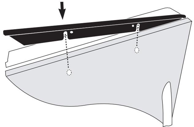
10. Fully seated top trim is close to flush with top of door and completely covers clips of side trim.
