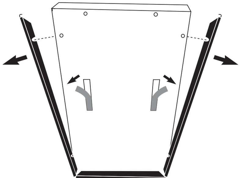
3. Align the bottom edge of the decorator panel to the lower fixed trim and center the panel with the door.
