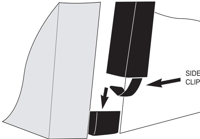
5. Rotate one piece of the side trim to seat into the decorator panel groove.
