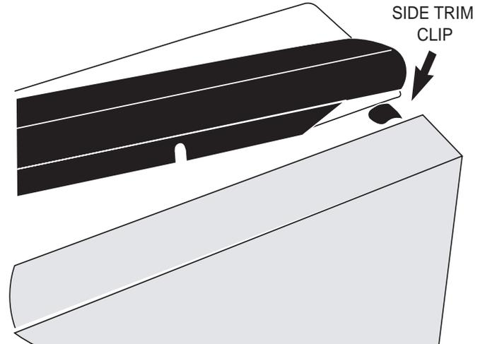
8. Assure the upper locking trim grooves engage the rivets on the door panel while simultaneously seating into the decorator panel groove.
