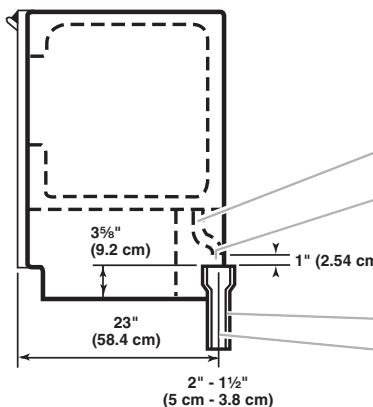
Drain lines must have a minimum of 5/8 in. (15.88 mm) inside diameter.
