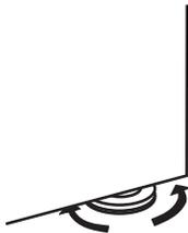
4. Open the door again and check to make sure that it closes as easily as you like. If not, tilt the refrigerator slightly more to the rear by turning both leveling screws to the right. It may take several more turns, and you should turn both leveling screws the same amount.
