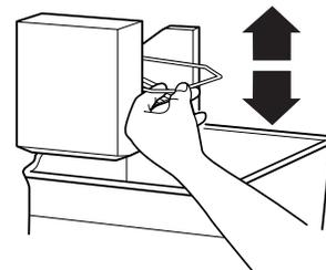
**NOTE:** Turn off the ice maker before removing the ice storage bin to serve ice or to clean the bin. This will keep the ice cubes from dropping out of the ice maker and into the freezer compartment. After replacing the ice storage bin, turn on the ice maker.
