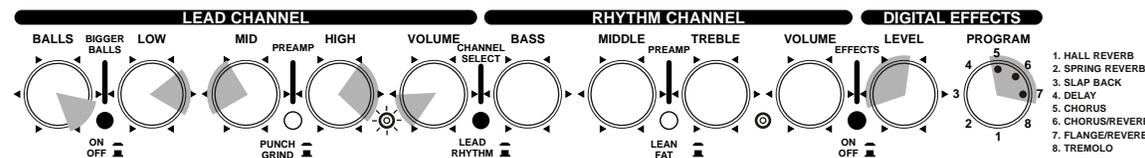
**Heavy Metal/Maximum Crunch** - this setting is a good starting point for the "notched out middle" sounds associated with metal and heavy alternative sounds. Adjust the Treble, Lows, Reverb and Chorus to taste. Usually, for a rhythm tone, you want to have more lower end and less for leads. Distortion is an integral part of this style of music and this amp delivers it quite well.
