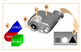
Infrared energy is emitted proportionally to the temperature of an object **A**. The warmer the object, the more energy it emits. The infrared energy from the objects is focused by the optics **B**, onto an infrared detector **C**. The information from the Infrared detector is passed to electronics **D** for image processing. The signal processing circuitry translates the infrared detector data into an image **E** that can be viewed on the built-in video monitor.
