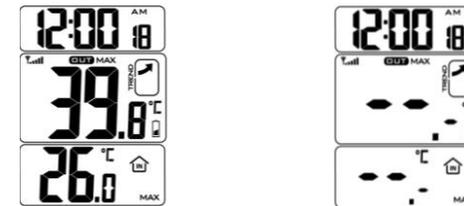
**VIEW MAXIMUM:** Press MAX/MIN key again, to show the maximum temperature records. In maximum memory display mode, **RESET MINIMUM:** With the maximum temperatures displayed, press and hold the MAX/MIN key for 2 seconds to manually clear the MAX records in memory.
