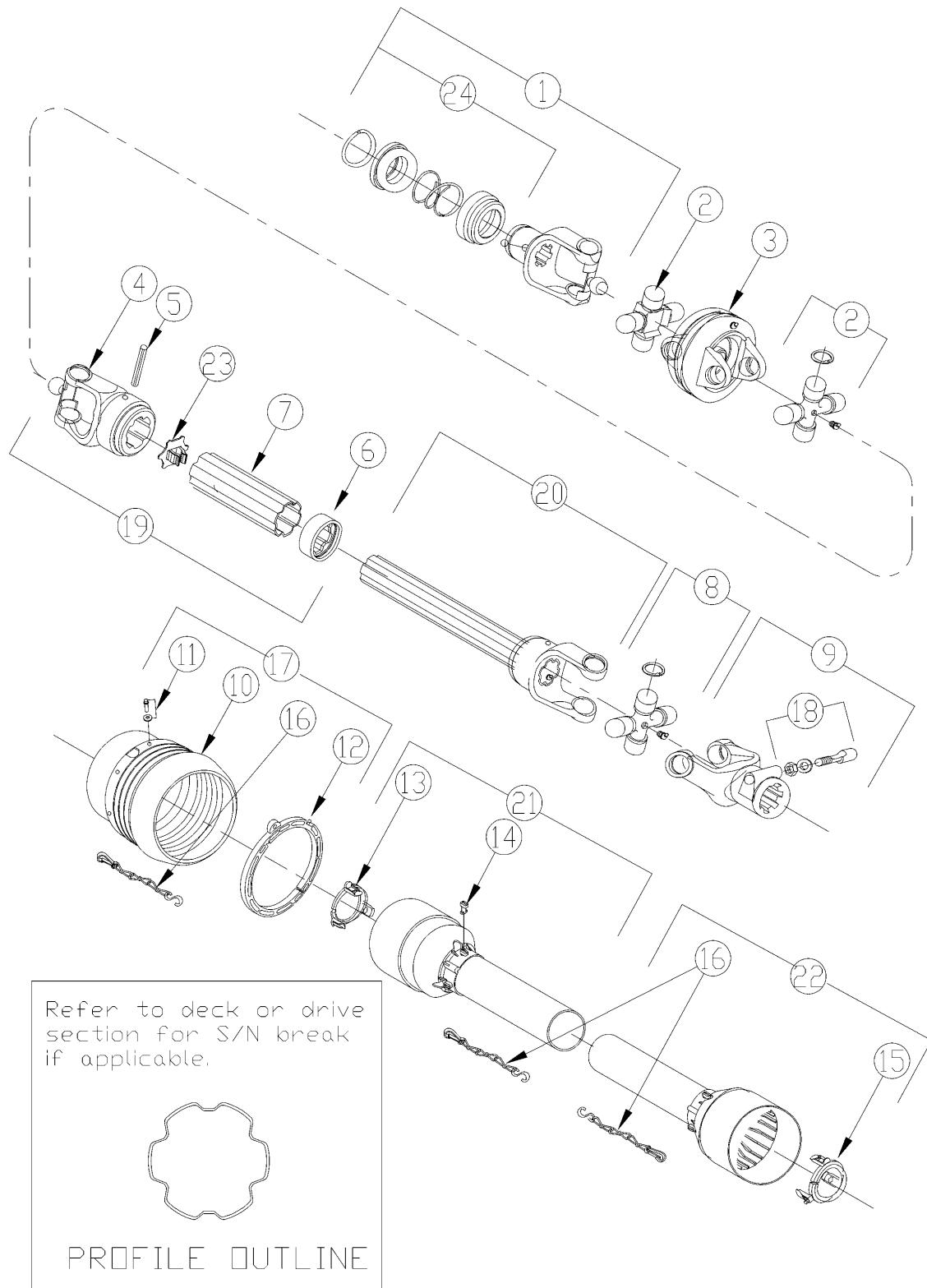
**Driveline CV 540 RPM (826-476C) Comer (S/N 468558 to \_\_\_\_\_)****Applies to RCB6010, RCB6015**
