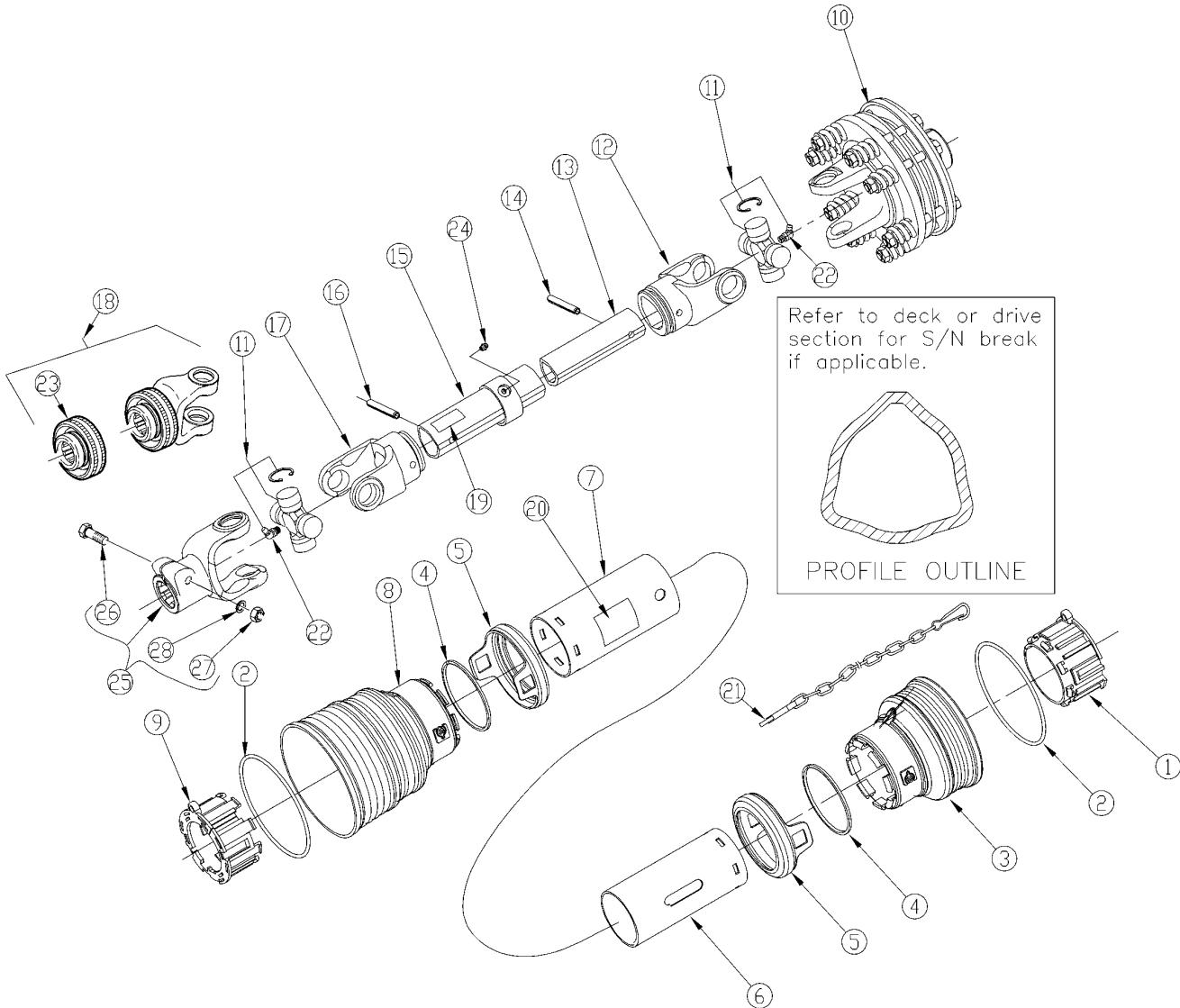
***Driveline Wing (826-185C) EC New Shielding*****Applies to RCB6010, RCB6015**
