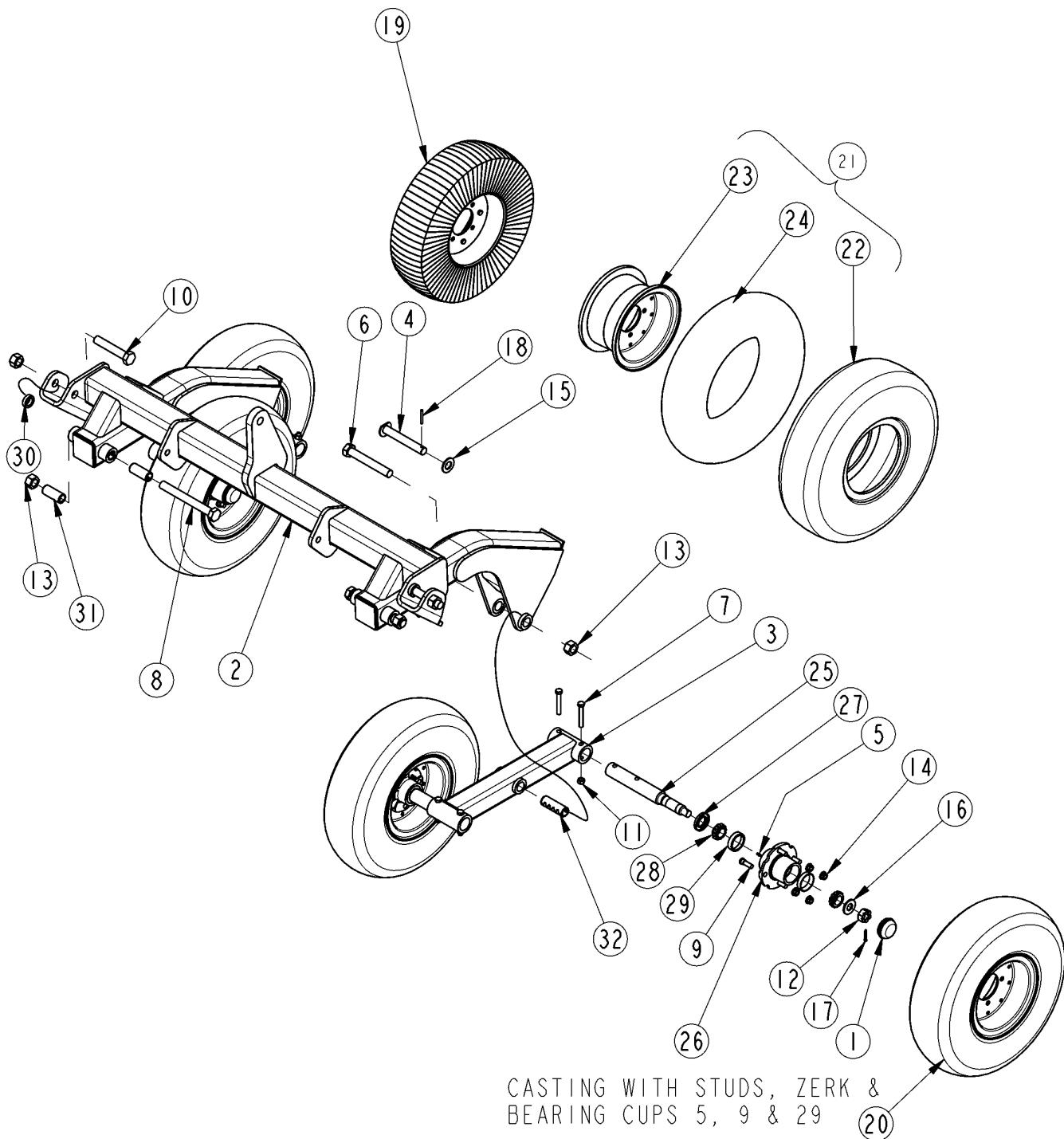
**Axle Tandem Center Deck (S/N 419602 to 489025)****Applies to RCB6010, RCB6015**
