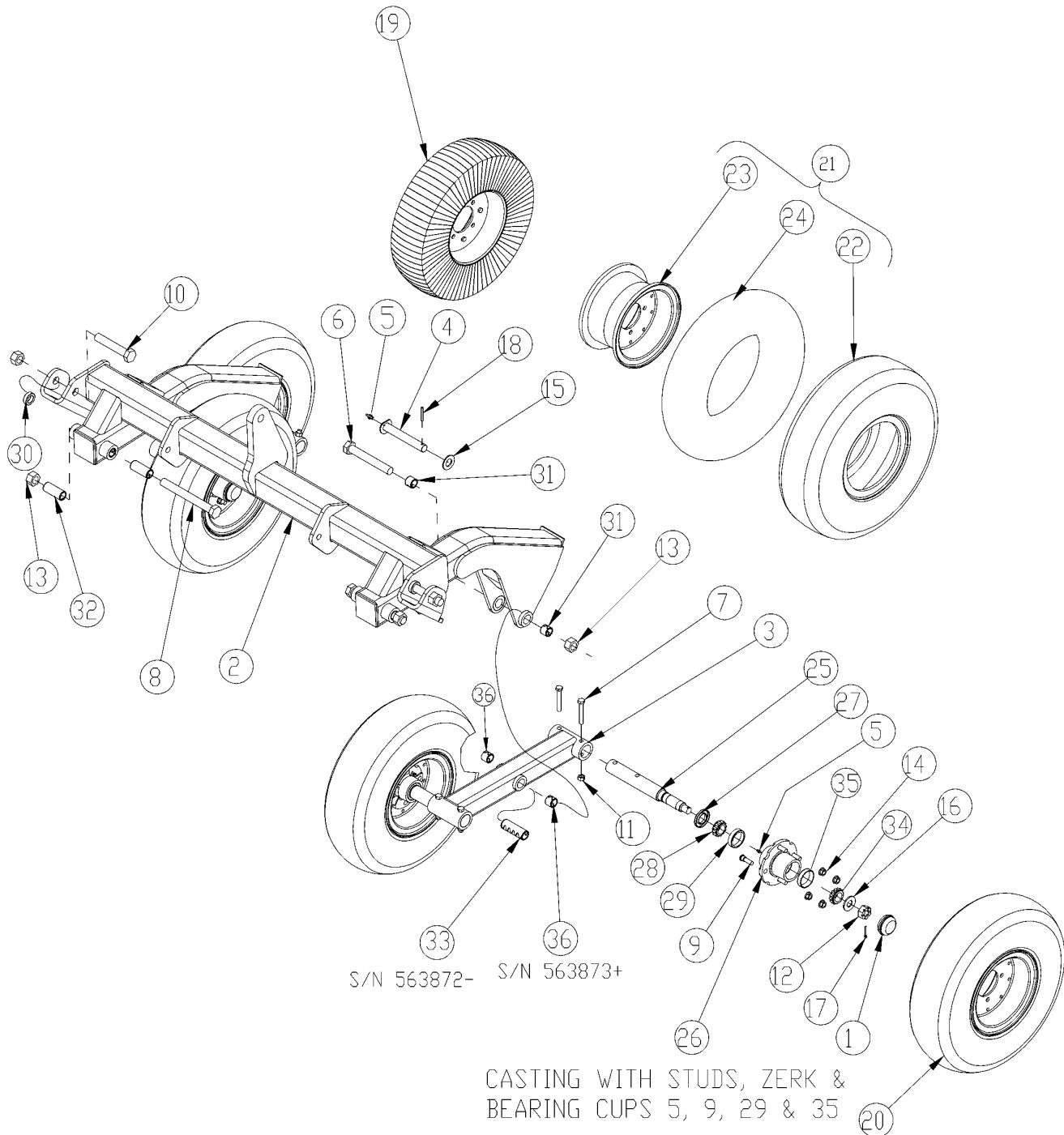
**Axle Tandem Center Deck (S/N 489026+)****Applies to RCB6010, RCB6015**
