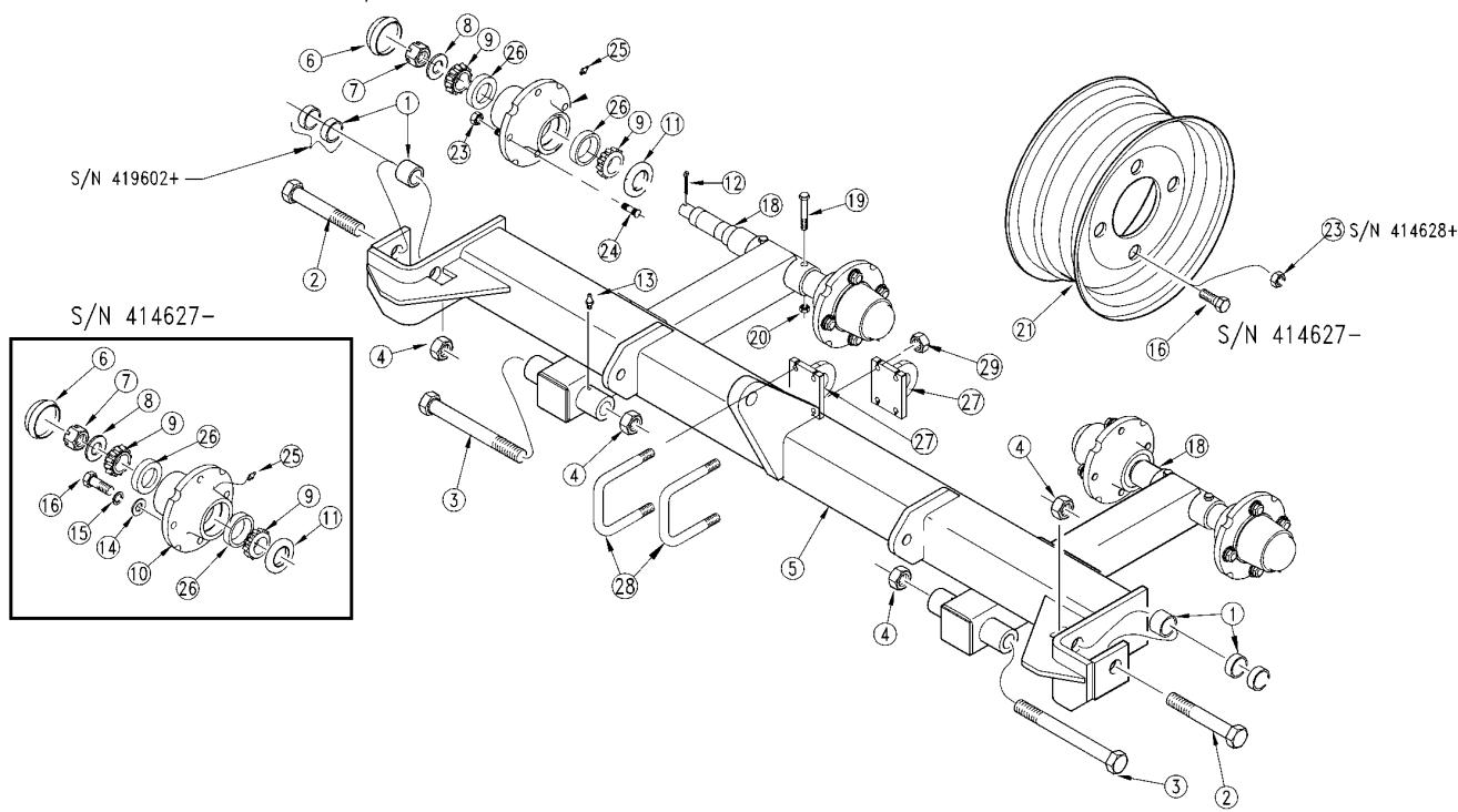
**Axle Center Deck (S/N 489025-)****Applies to RCB6010, RCB6015**
