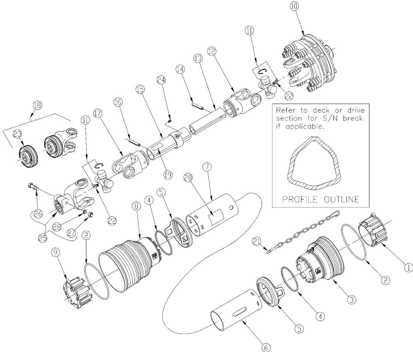
**Driveline Wing (826-185C) EC New Shielding****Applies to RCBM6010, RCBM6015**
