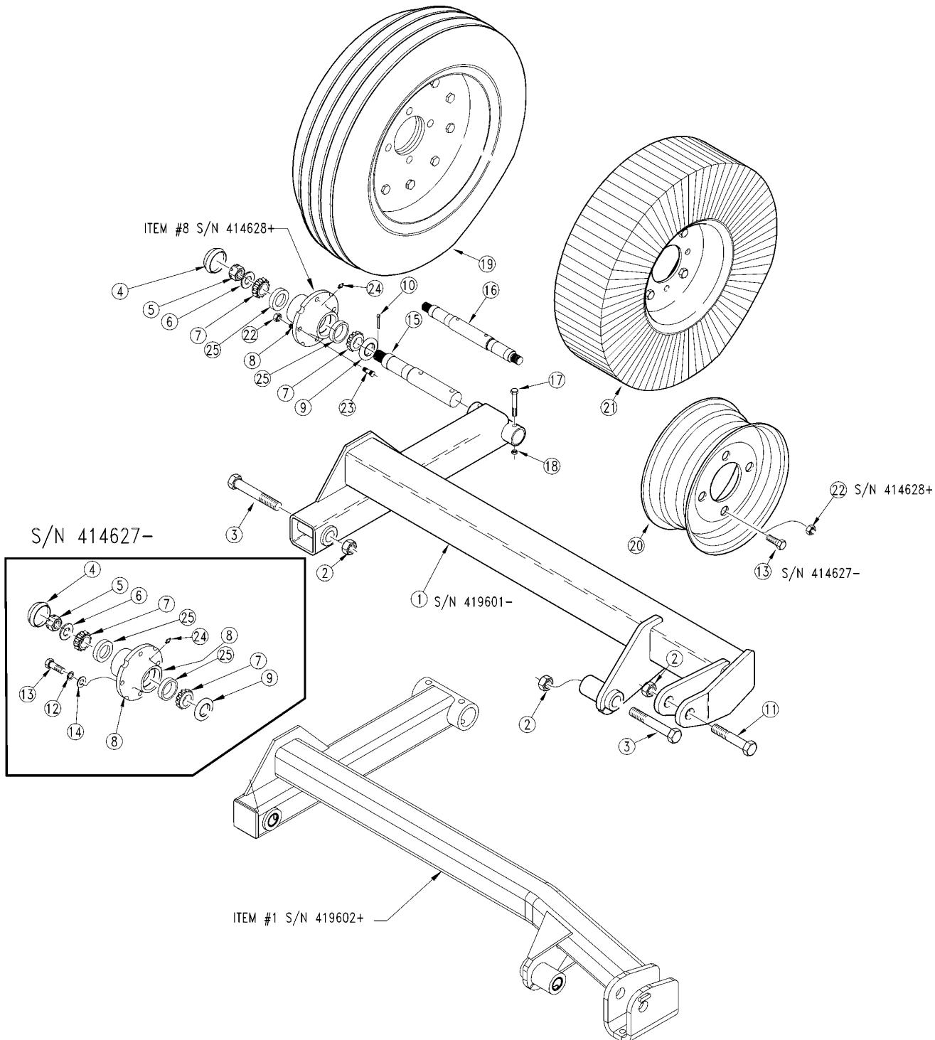
**Axle Wing Deck (S/N 489025-)****Applies to RCB6010, RCB6015**
