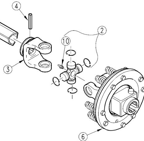
***Driveline Center 540 RPM (826-183C) Eurocardan*****Applies to RCB6010, RCB6015**
