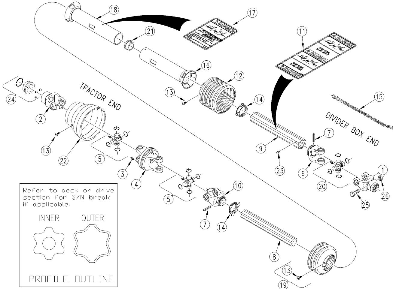
**Driveline CV 1000 RPM (826-245C) 1 3/4-20 Walterscheid (S/N 488896-)****Applies to RCBM6010, RCBM6015**
