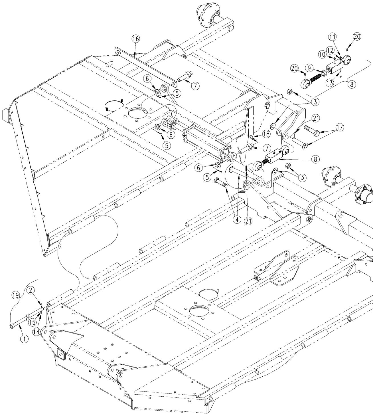
**Wing Turnbuckle and Transport Bar****Applies to RCB6010, RCB6015**
