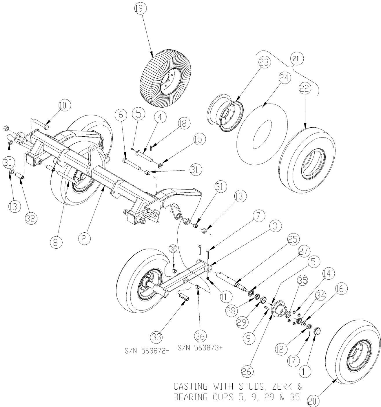
**Axle Tandem Center Deck (S/N 489026+)****Applies to RCBM6010, RCBM6015**
