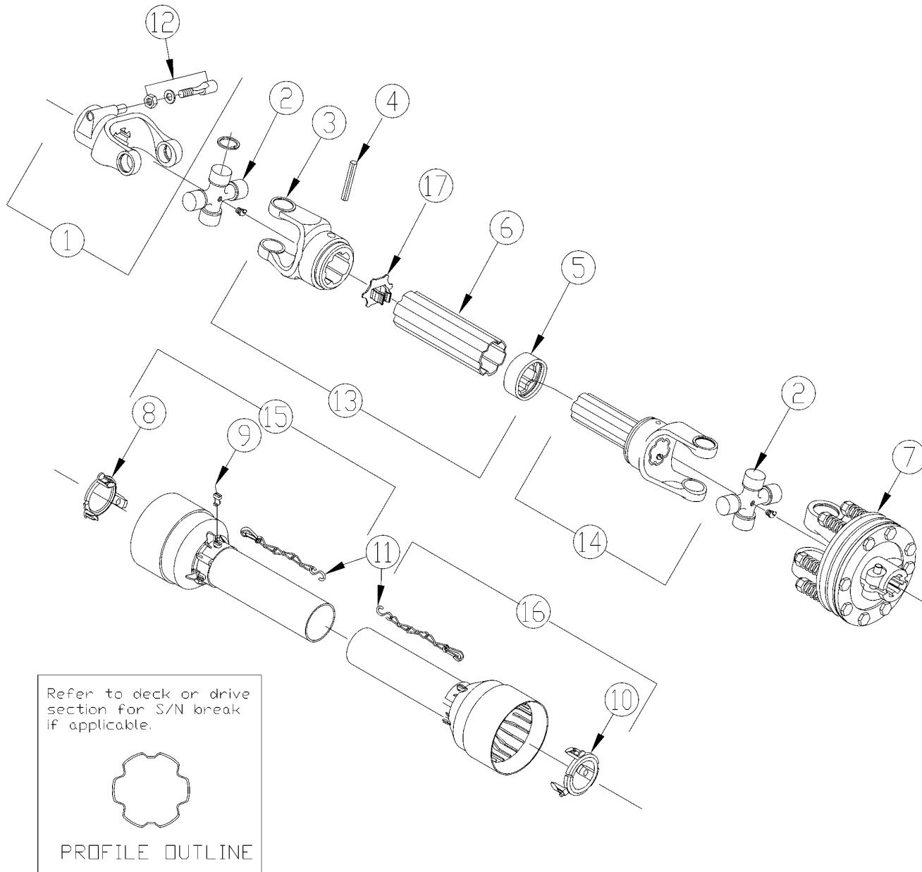
**Driveline Wing (826-481C) Comer (S/N 461935 to 461937, 468573+)****Applies to RCBM6010, RCBM6015**
