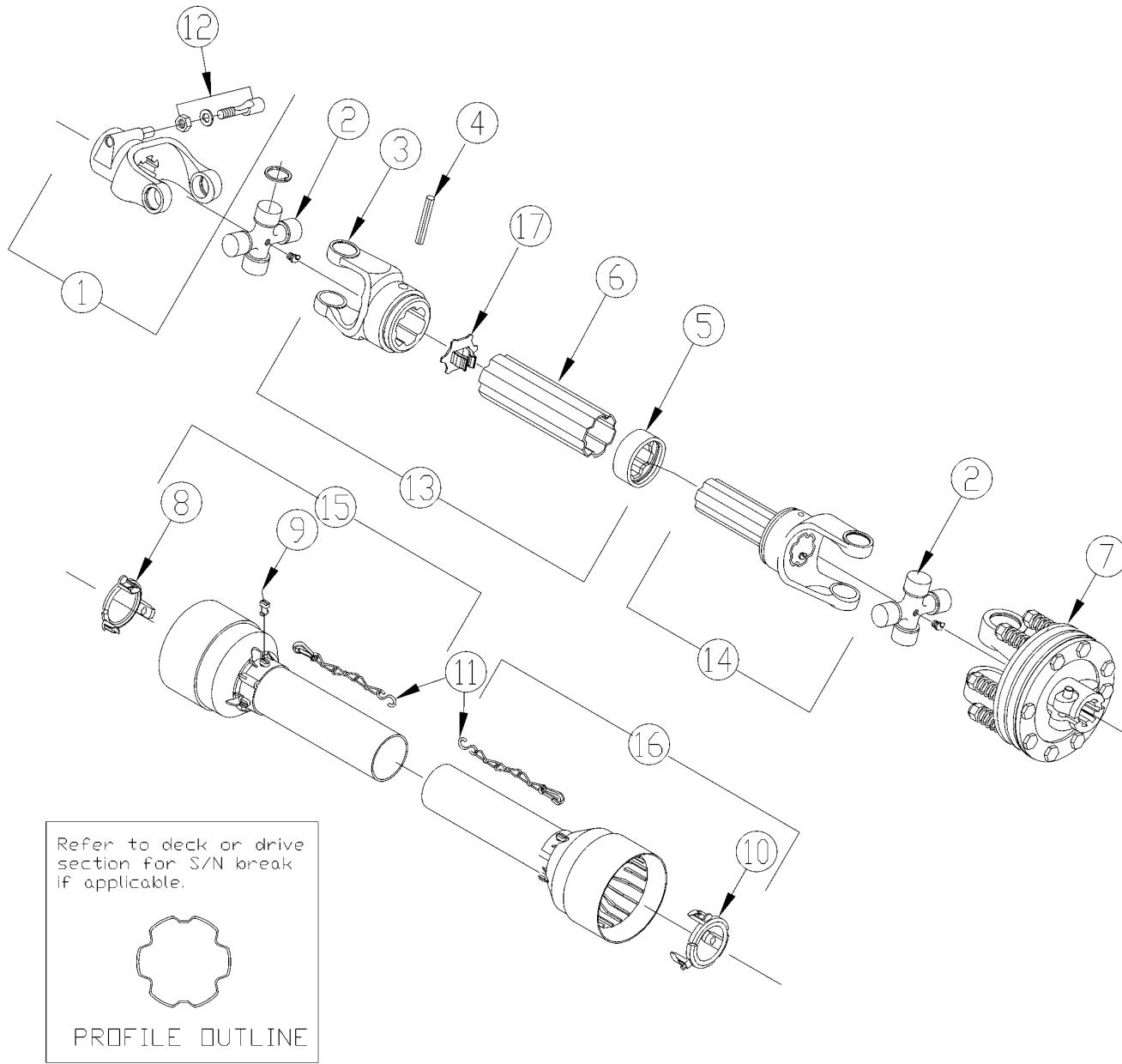
***Driveline Wing (826-481C) Comer (S/N 461935 to 461937, 468573+)*****Applies to RCB6010, RCB6015**
