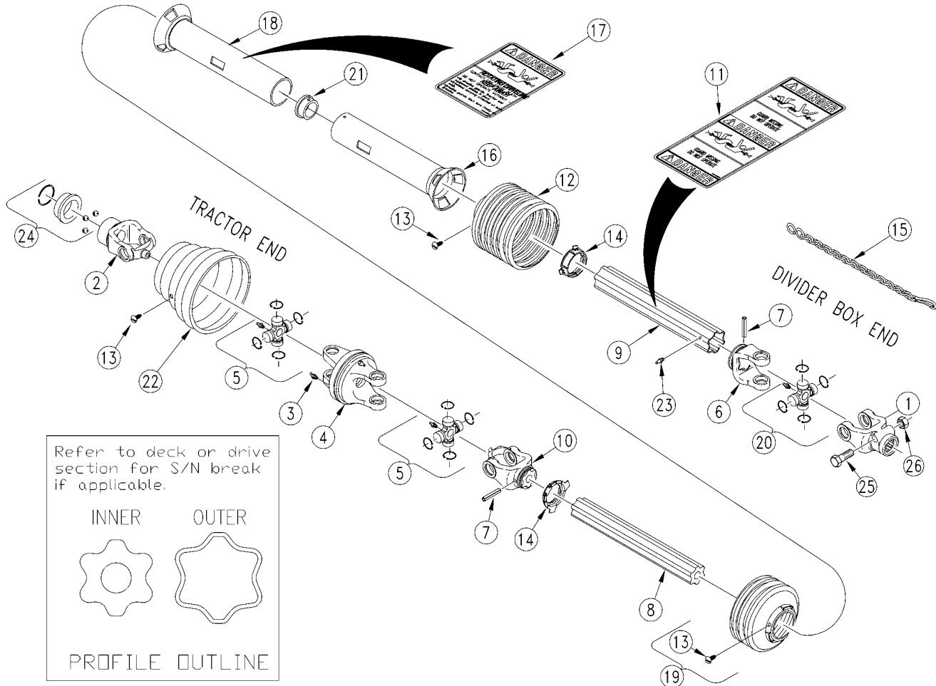
***Driveline CV 1000 RPM (826-244C) Walterscheid (S/N 468225-)*****Applies to RCBM6010, RCBM6015**
