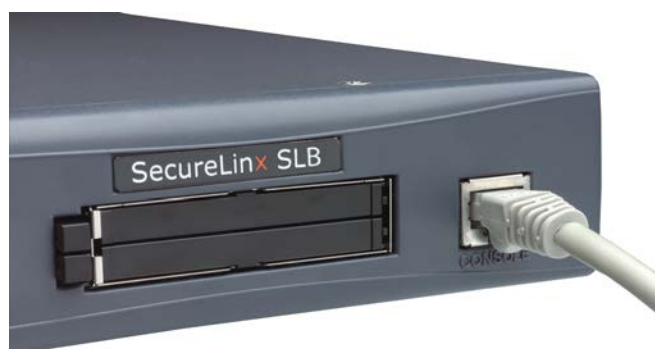
Figure 2-4. Console Port Connection
