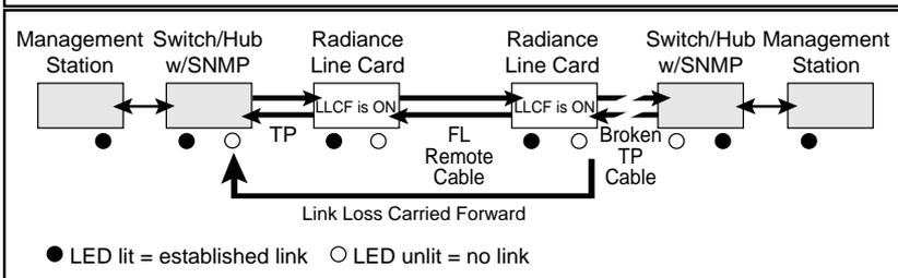
**Important:** When connecting a Radiance line card with LLCF enabled to an auto-negotiating device, force both sides of the configuration to 10Mbps and either full or half duplex. This allows the card to immediately see link pulses and start passing data.
