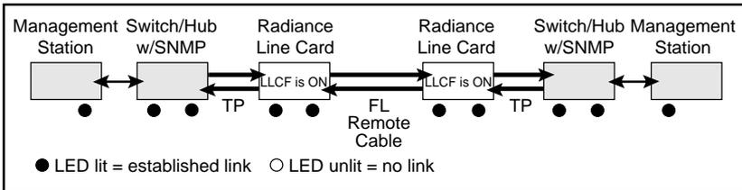
If the connection breaks, the line card carries that link loss forward to the switch/hub which generates a trap to the management station. The administrator can then determine the source of the problem.
