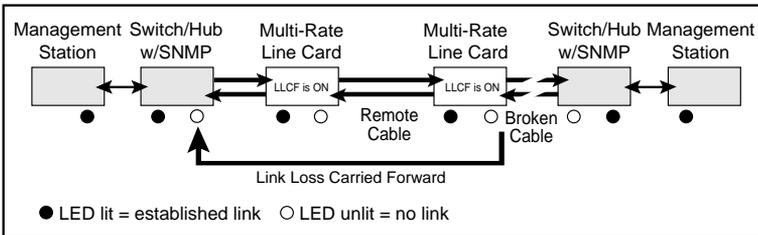
**NOTE:** Loopback takes precedence over LLCF. If LLCF and loopback are both enabled, LLCF functionality will be ignored for the port that is in loopback. LLCF will remain in effect for the port that is not in loopback.
