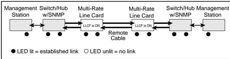
If a connection breaks, the line cards will carry that link loss forward to a switch/hub which generates a trap to the management station. The network administrator can then determine the source of the problem.
