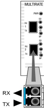
**IMPORTANT:** The multi-rate line card is designed and tested to operate using only Metrobility-supplied SFP transceivers. Safety, performance, and reliability are guaranteed only when Metrobility-supplied transceivers are used. **Installing unspecified parts may damage the product and will void the unit's warranty.**
