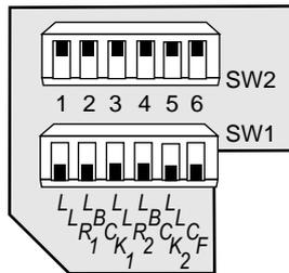
When setting DIP switches\*, the UP position is when the lever of the switch is pushed away from the circuit board. The DOWN position is when the lever of the switch is pushed toward the circuit board.
