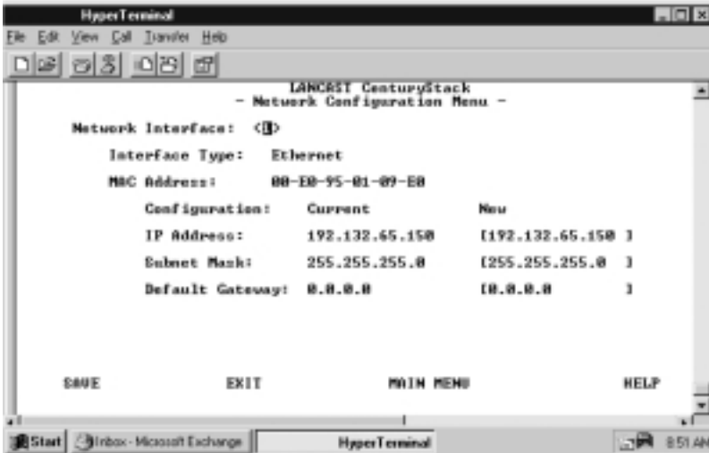
In-Band Ethernet Configuration Menu
