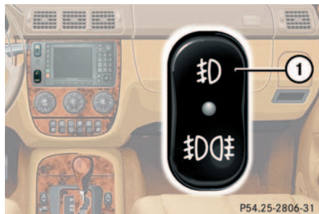
1 Switch for fog lamps
