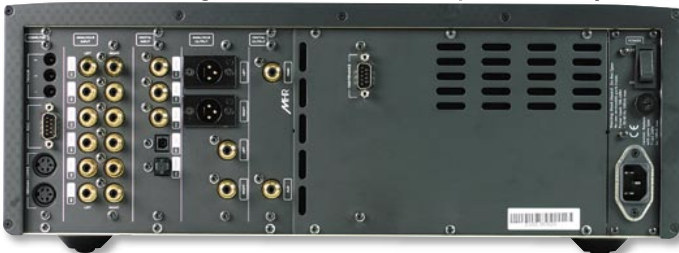
808i (Player/Preamplifier model) Rear Panel. The 808 Player model does not include the analogue and digital input panel areas.
