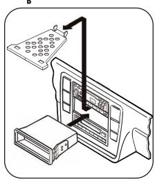
Note: This installation kit is an extremely tight fit and requires force to be "snapped" into the dash opening. Removal of aftermarket radio is even more difficult than installation, so please be sure to fully test the aftermarket radio prior to completing the kit's installation.
