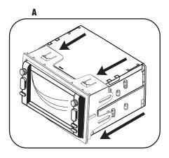
Note: This installation kit is an extremely tight fit and requires force to be "snapped" into the dash opening. Removal of aftermarket radio is even more difficult than installation, so please be sure to fully test the aftermarket radio prior to completing the kit's installation.
