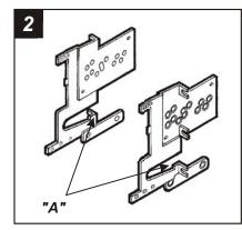
Locate the corner of each lower mounting tab on the *Mounting Brackets* ("A").
