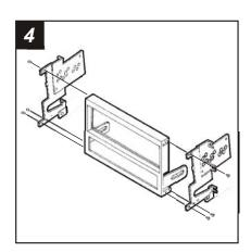
Align the OUTER holes in the *Mounting Brackets* with the holes in the *Radio Housing* and mount with *(6) #6 Self-tapping Screws* supplied. (The Brackets will mount on an angle). *Skip to the Installation Instructions for ALL VEHICLES on Page #3.*
