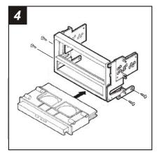
Remove (4) screws securing the cupholder to the factory head unit assembly and remove. Slide the cupholder into the bottom of the *Radio Housing* and mount with the same (4) screws. Skip to the Installation Instructions for ALL VEHICLES on Page #3.
