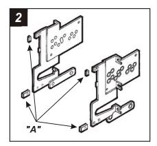
Using the raised lines as a guide, cut and remove the ends of each *Mounting Bracket* ("A").
