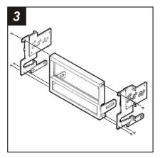
Align the holes in the *Mounting Brackets* with the holes in the *Radio Housing* and mount with (6) #6 Self-tapping Screws supplied.
