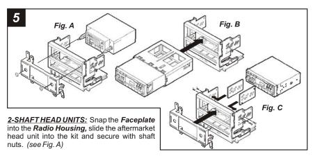
**DIN HEAD UNITS:** Slide the DIN cage into the Housing and secure by bending the metal locking tabs down. Slide the aftermarket head unit into the cage until secure. (see Fig. B)
