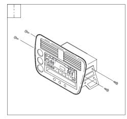
Remove (4) Phillips screws from each side securing the factory head unit to the bracket assemb yand remove the unit.
