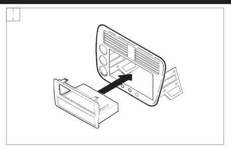
Snap the Radio Housing nto the sub-dash.
