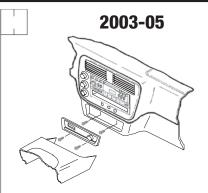
Unsnap and remove trimring from around foor shifter. Unsnap and remove arger trim around floor console shifter. Remove (2) phillips screws from in between cupholder and shifter. Unsnap sides of console (2 snaps per side) and remove with power outlet assembly. Remove (2) phillips screws from under radio assembly, facing up.
