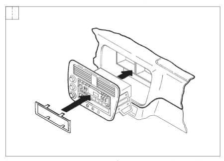
Re-connect the battery terminal and test the unit for proper operation. Snap the *Trimplate* over the mounted head unit. Slide the dash trim bezel assembly into the sub-dash until secure.
