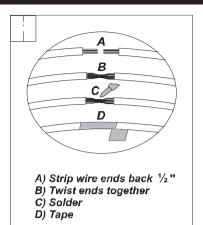
Locate the factory wiring harness in the dash. Metra recommends using the proper mating adaptor and making connections as shown. (Isolate and individually tape off the ends of any unused wires to prevent electrical short circuit).
