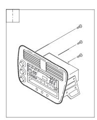
Remove (3) screws securing the climate control pod to the back of the dash trim bezel and remove the pod.
