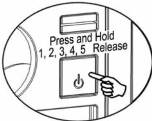
Figure 16: Laser & Motor Off Power Save Mode
