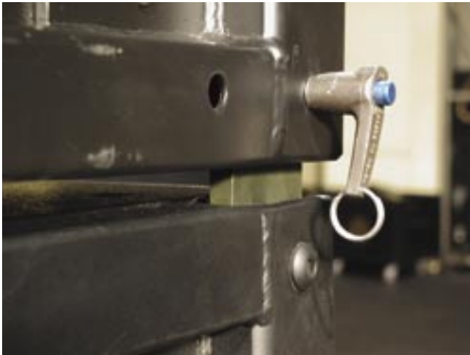
Figure 27. Rear link QRP inserted
