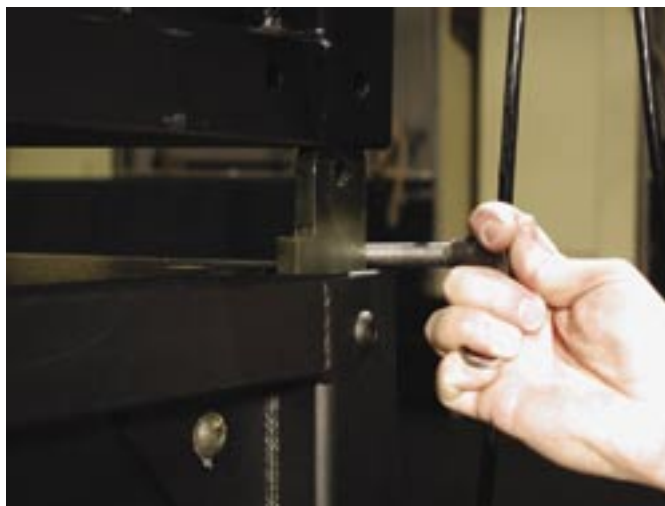
Figure 25. Holding the rear link using a QRP
