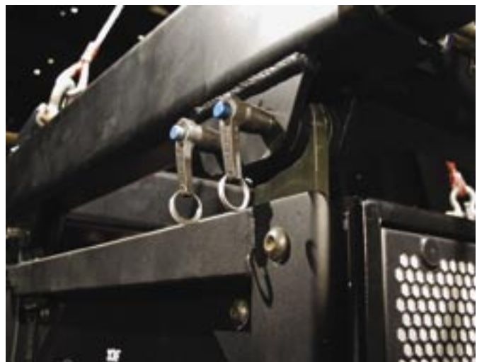
Figure 16. The QRP securing rear link in retracted position
