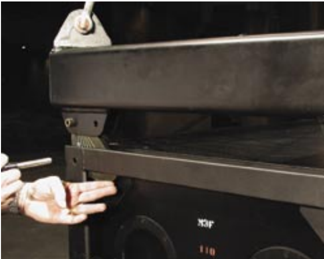
Figure 19. Removing the QRP from the MTG-3D Top Grid's front CamLink
