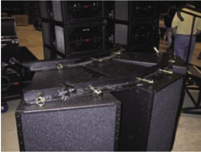
Figure 44. Transition frame with downfill loudspeakers
