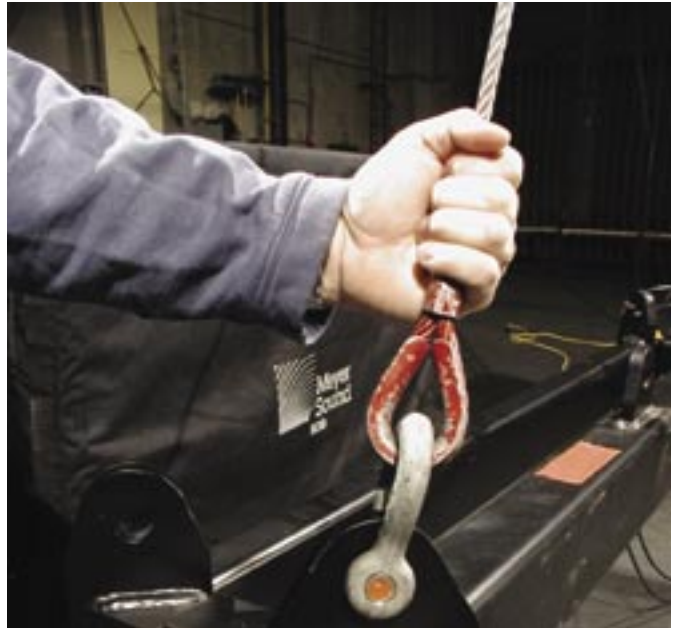
Figure 12. Attaching motors or bridle legs to the MTG-3D Top Grid
