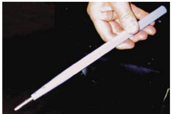
Figure 30. 0.25" (6.35 mm) drift punch
