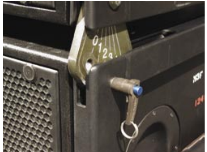
Figure 29. QRP fully inserted into 3° hole
