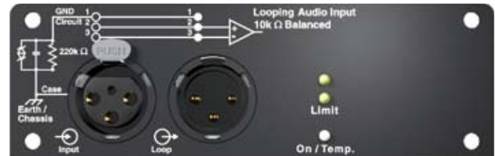
Figure 3.1. Side panel audio input connectors
