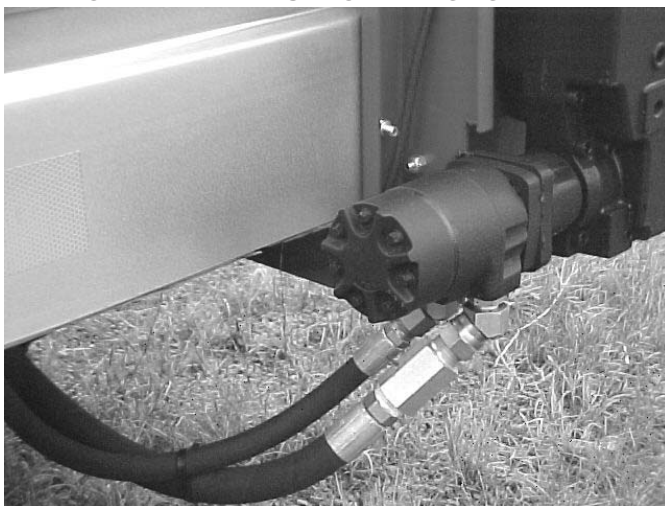
HYDRAULIC CHECK VALVE AT REAR OF BOX
